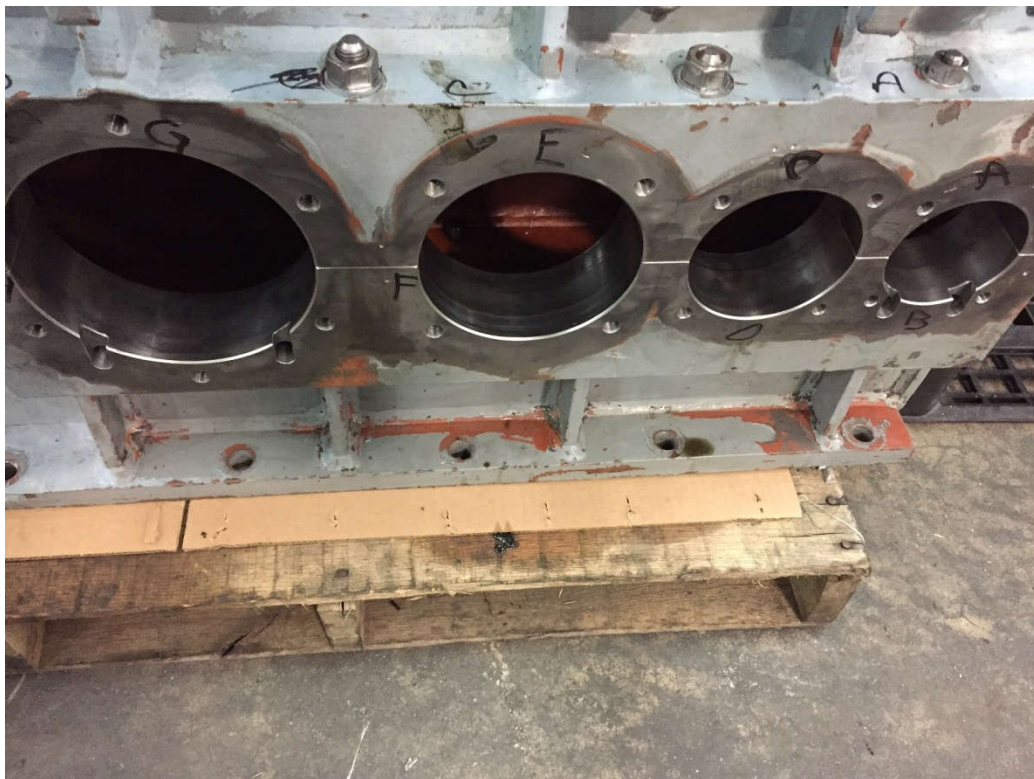
DE side of the gearbox housing
