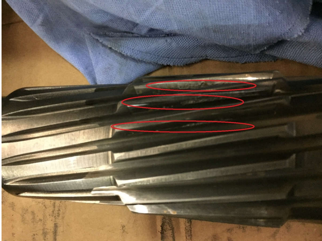
Worn and pitted teeth of second reduction pinion
