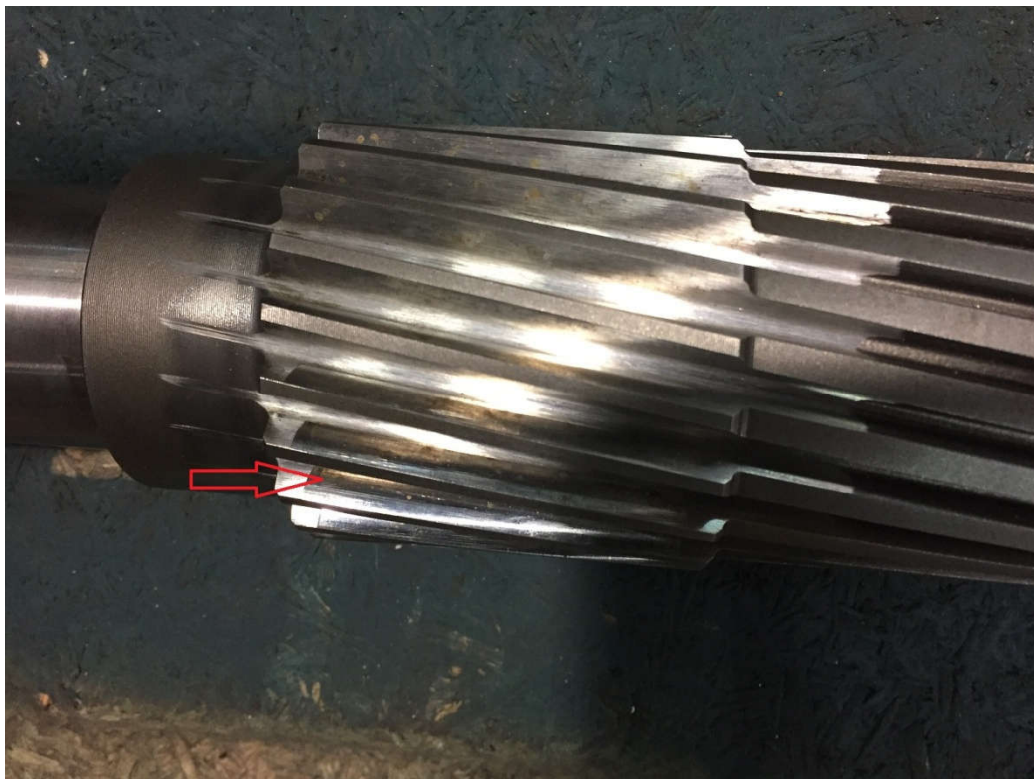
Worn teeth of first reduction pinion
