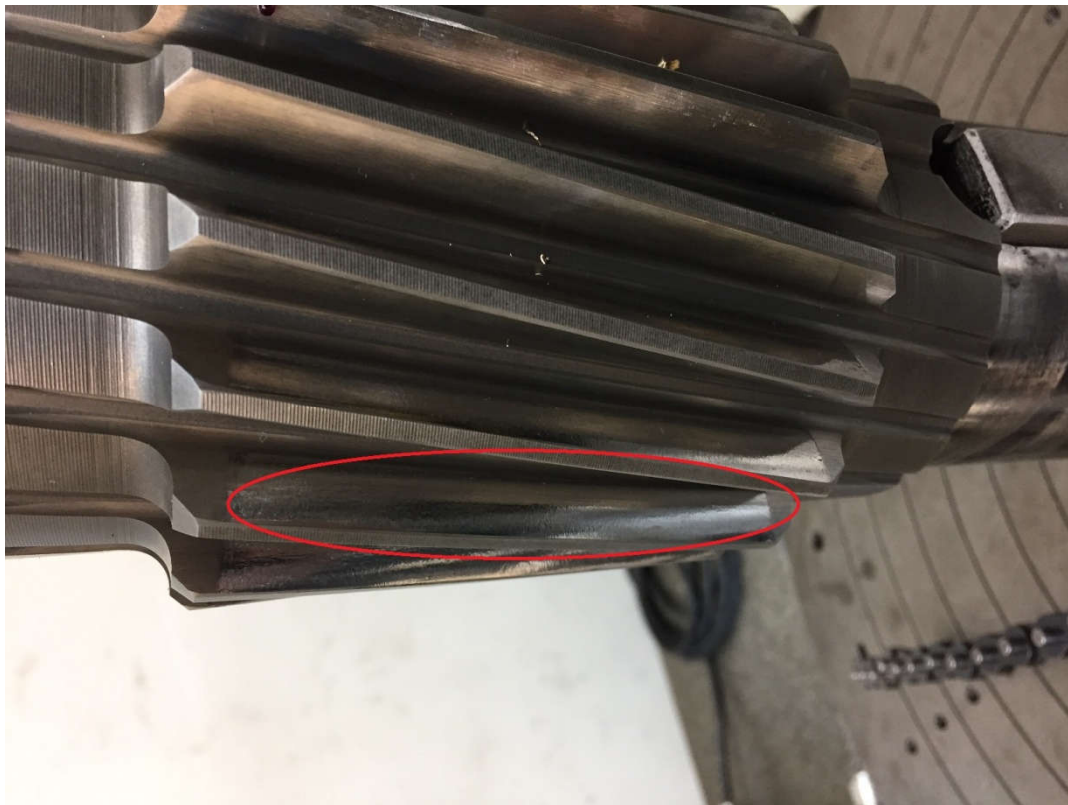
Worn teeth of low-speed pinion
