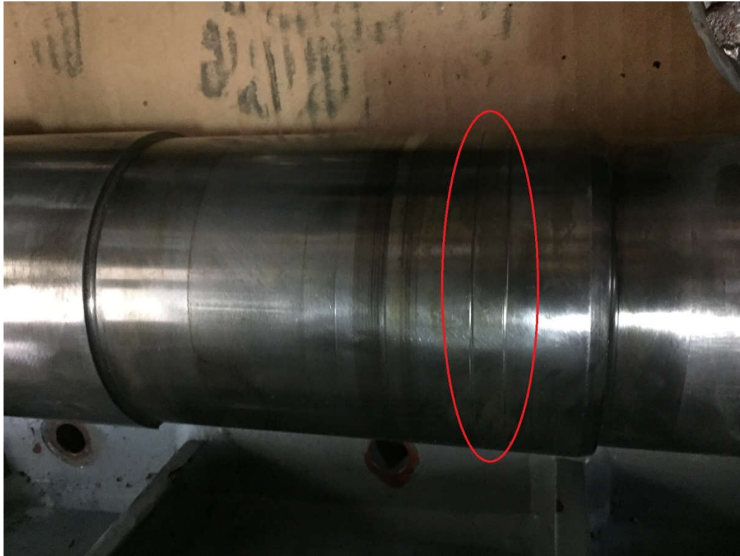
Damaged seal area on output shaft
