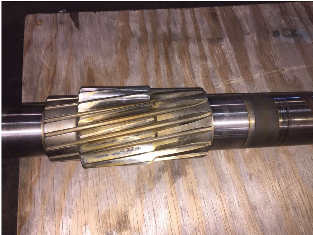
High-speed pinion with damaged seal area
