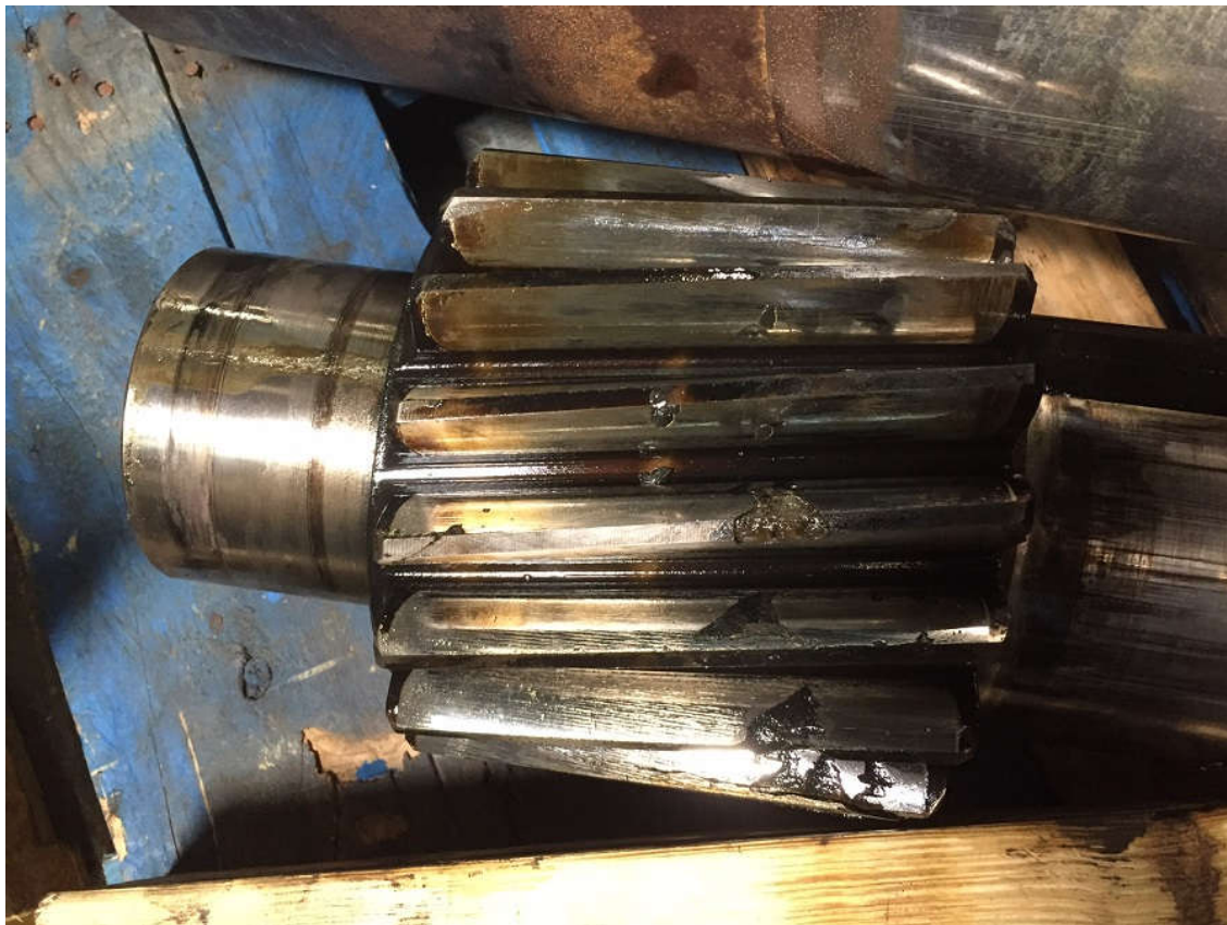
Damaged low-speed pinion
