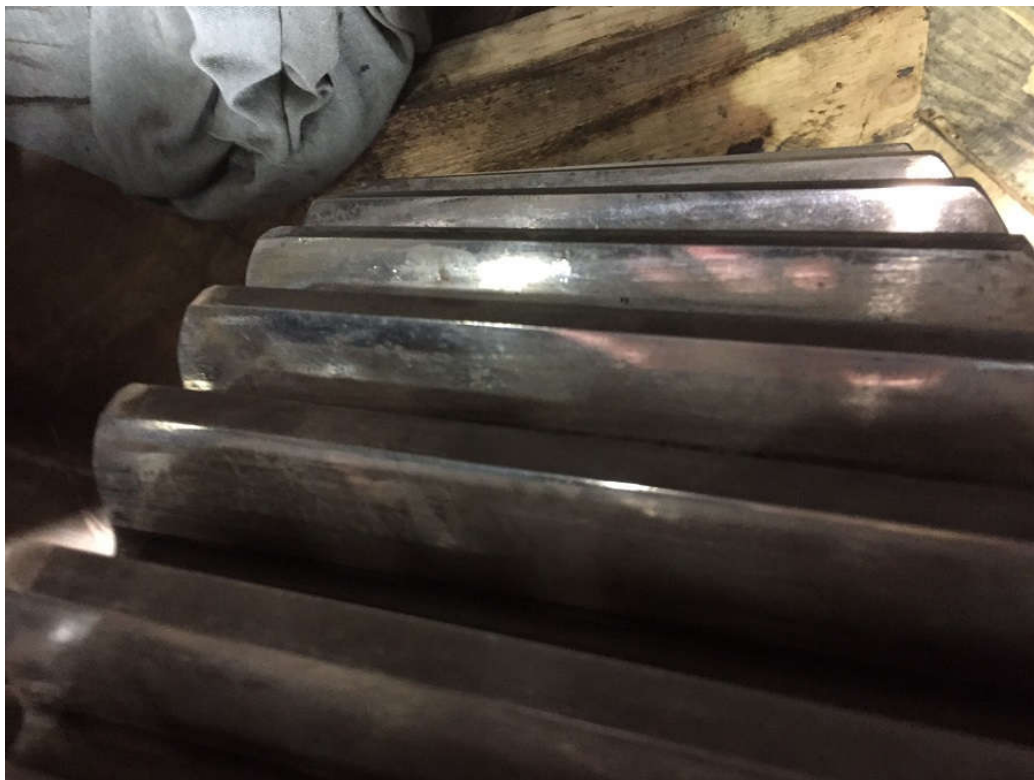
Heavily pitted and worn low-speed gear
