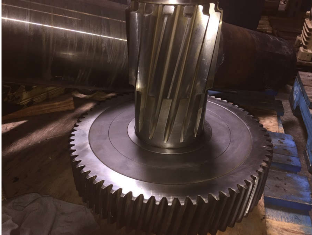
2 nd reduction pinion and high-speed gear in good condition
