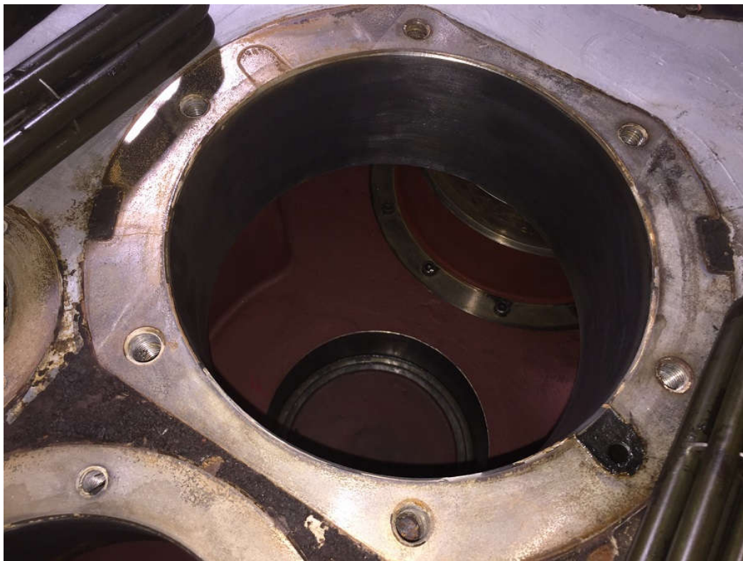
Damaged low-speed pinion bore
