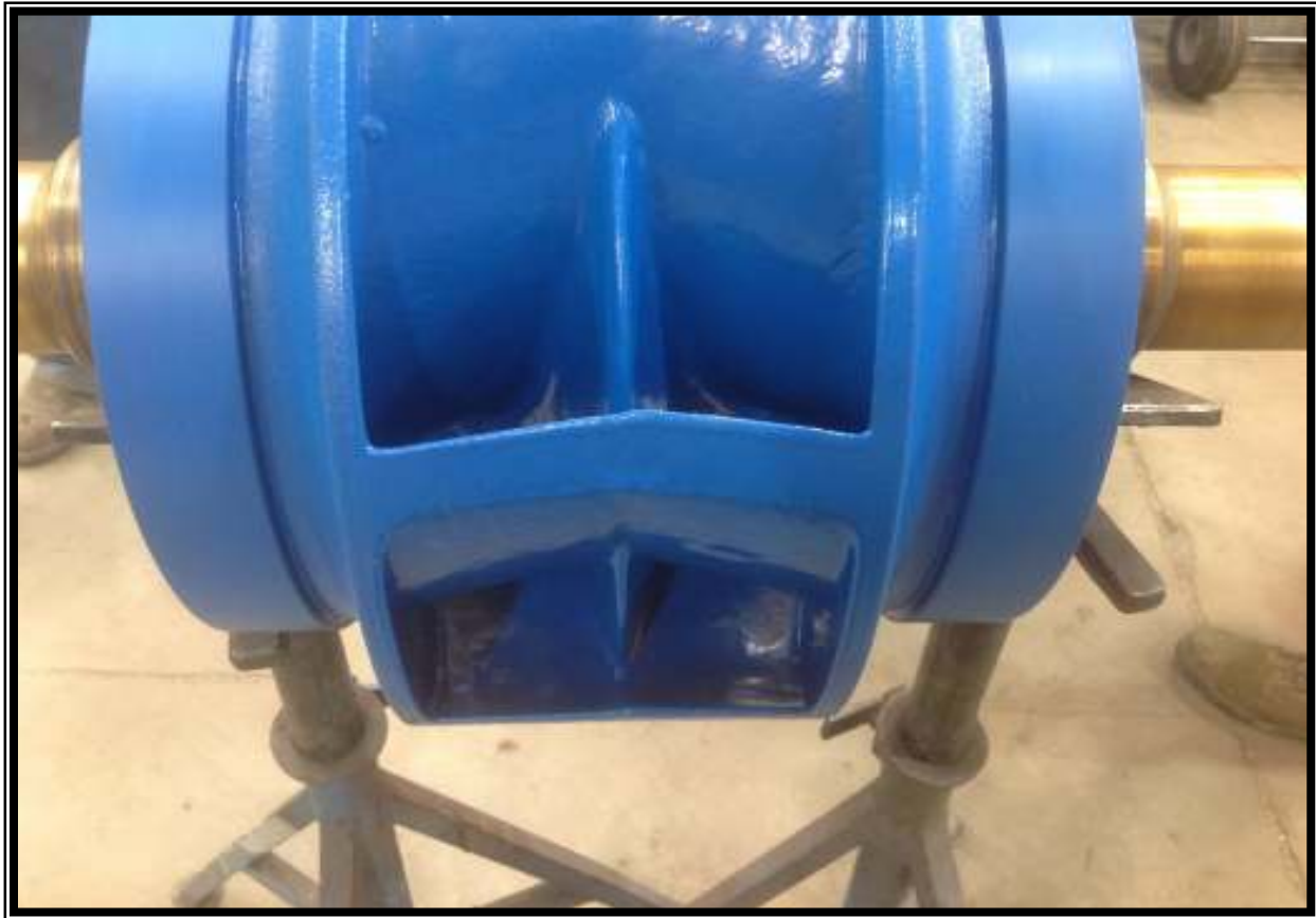
Photo 1 : #2 High Service Pump - Rotating Assembly
